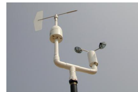
A portable weather station is used at scene by HKO to assess downwind conditions.
